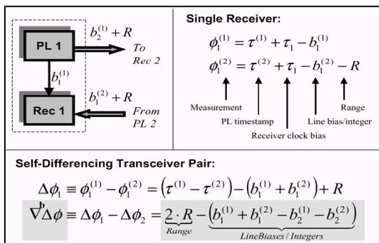
Fig. 5 Double differencing with transceivers (LeMaster, 2002)
