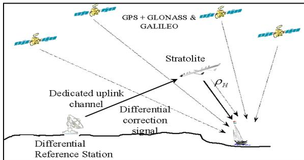
Fig. 1 Differential satellite positioning with a stratolite (<http://www.helinet.polito.it>)
